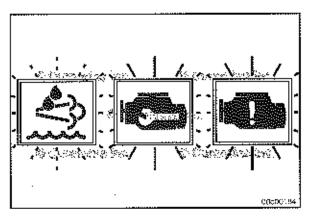
If the engine has been shut down or has idled for an extended period of time after the DEF tank has been emptied, the STOP ENGINE lamp will also be illuminated along with the flashing AFTERTREATMENT DIESEL EXHAUST FLUID lamp and illuminated CHECK ENGINE lamp. The engine power will continue to be limited automatically. The vehicle speed will also be limited to 5 mph.
