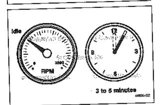
Idle the engine for 3 to 5 minutes before operating with a load.
