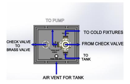
**DRY CAMPING**- TO RUN HOT AND COLD FIXTURES FROM STORAGE TANK (VIA RV PUMP)
