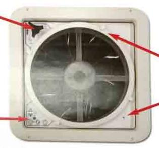
With the fan motor running, close the Vent Lid to enter Ceiling Fan. Mode. The fan motor will continue to run and circulate air within the RV cabin.
